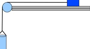
Slowly, while holding the cup, add one nut at a time to the cup and test it to see if there are enough nuts to pull the bock along the flat surface. Once you have enough nuts, weigh them.
